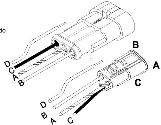
(A) RED: Power - Connect to power (+10-30VDC) through your switch using a 5 amp fuse.
